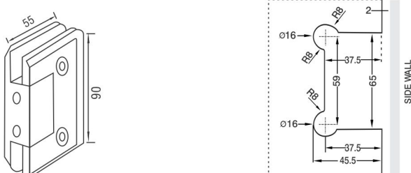
Size & Cutout Details for TCH-8430 & TCH-8437 Wall to Glass 90° Fix Bracket
